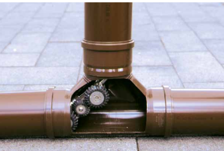
The double swept angle of the T-Section base unit provides easy access for CCTV-Cameras in both directions.
