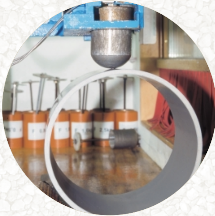
Impact test in accordance with EN 744 at 0°C
